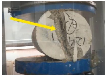
Fig 5 Typical splitting tensile failure mode patterns
